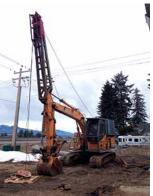
1996 CASE 9030B EXCA-LINER Excavator has a Cummins 6BT 5.9, Set up with LS98
