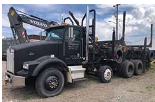
1987 KENWORTH T800 MULE TRAIN Cummins BC4 450hp, 15 speed, Eaton DT402 two speeds 4.11/5.61, on walking beam suspension, with 1982 Utility pup, 8'6" bunks with Vulcan scales, 85% tires, 28,500 empty weight, $30,000. Call 509-535-4427 Spokane
