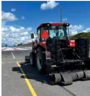
The tractor used to apply rubber to the track in order to improve traction and the view from the driver's seat.
