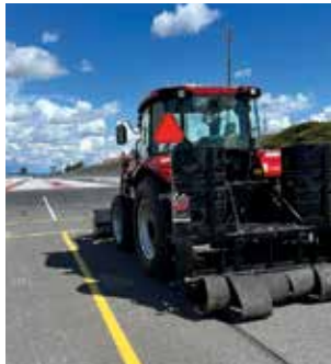
The tractor used to apply rubber to the track in order to improve traction and the view from the driver's seat. Qlipse Raceway photos
