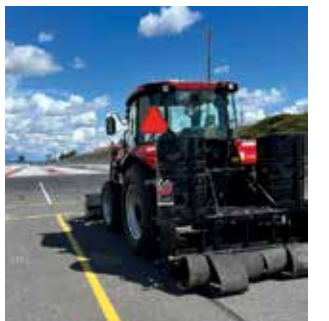
The tractor used to apply rubber to the track in order to improve traction and the view from the driver's seat.
